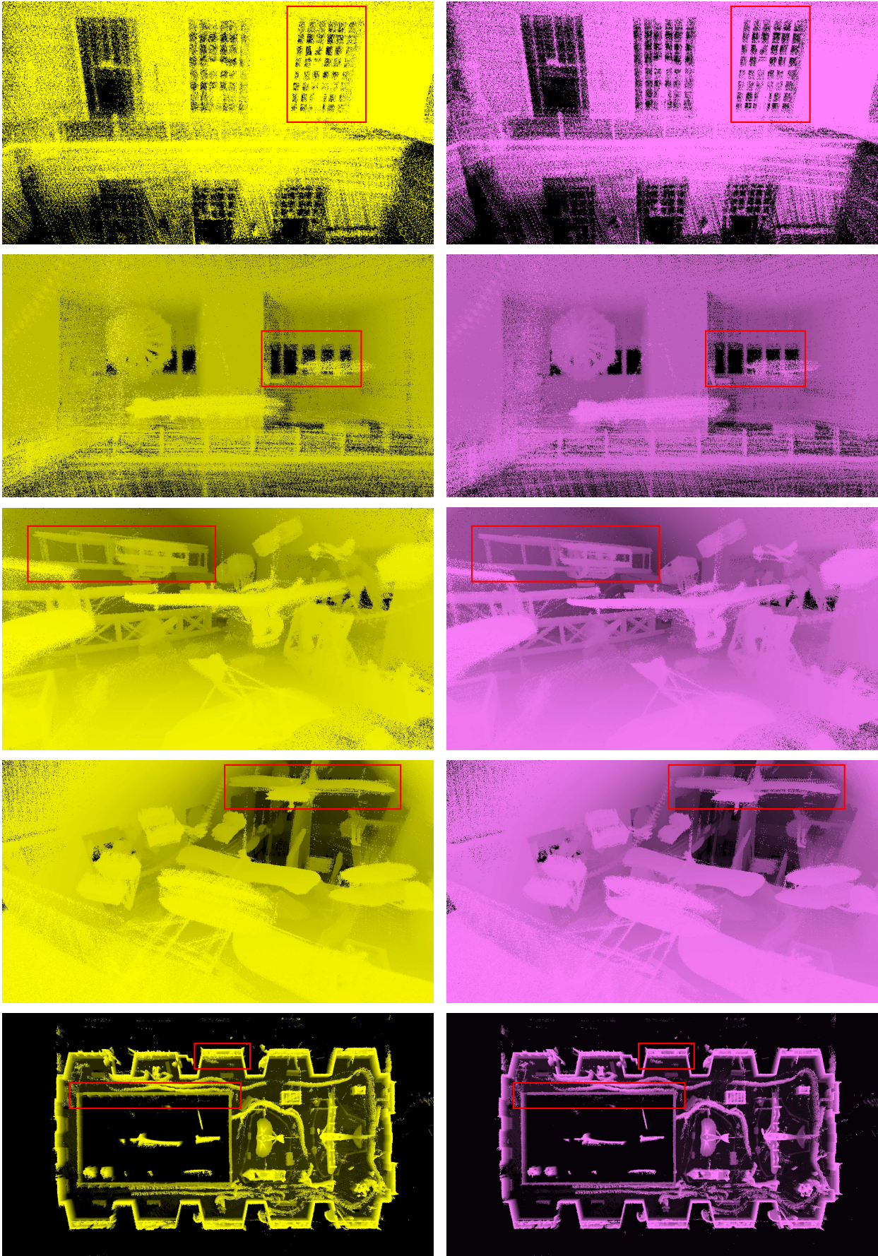
Figure 3: Results of continuous-time SLAM on Google’s Cartographer sample data set Deutsches Museum in München. Left: input. Right: output of our solution. Shown are 3D views (perspective) of the scene. Major changes in the point cloud are highlighted in red. Continued in Figure 4
