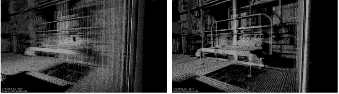
Figure 4: Left: Before applying our semi-rigid SLAM method. Right: Correction by our semi-rigid SLAM.
