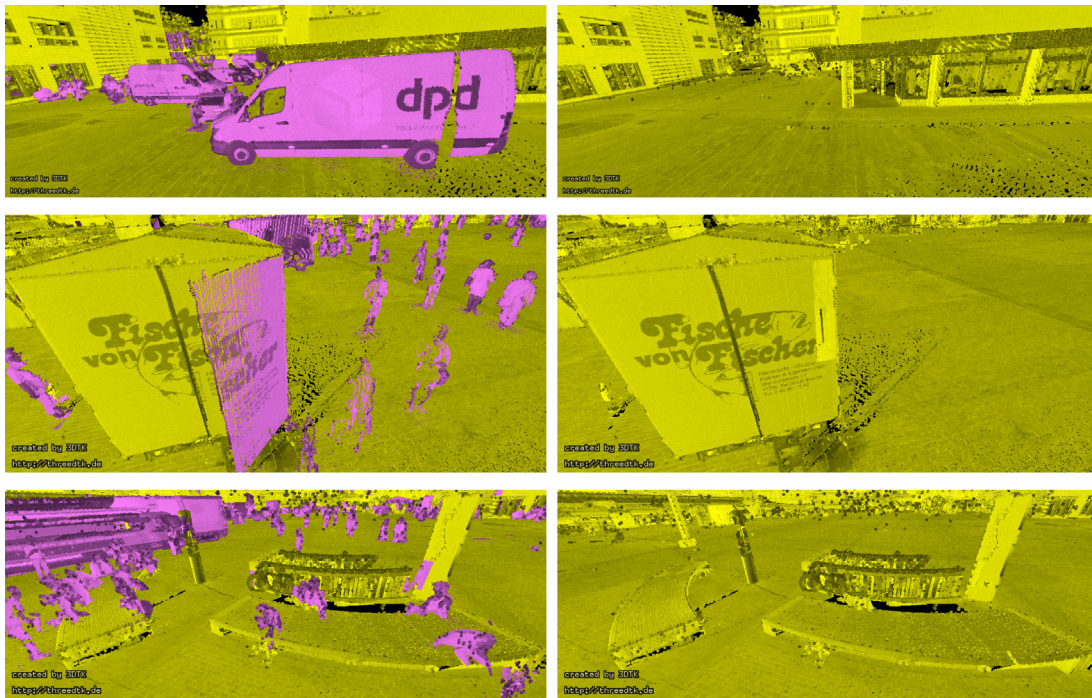
Fig. 24. Würzburg city dataset: Each row shows the same camera position. Left column: Static points in yellow and dynamic points in magenta. Right column: scene with only static points. (For interpretation of the references to color in this figure legend, the reader is referred to the web version of this article.)
