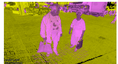
Figure 3: Non-static points are identified (magenta)...
