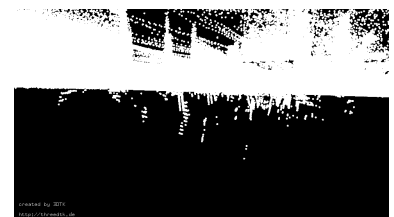
Figure 4.35: Points from reflections under the street surface
