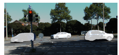
Figure 4.36: Examples of wrong classifications of binary masks from FuseMODNet from KITTI scene 9, frame 385.
