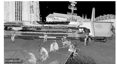
Figure 2: A "stretched" van from the Würzburg dataset due to the vehicle moving in the direction of the scanner rotation in a terrestrial mapping scenario
