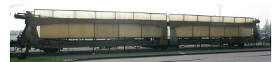
Figure 3.15: A photo of the scanned train wagon with a bogie distance of 20 m.
