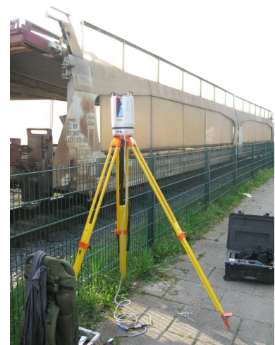
Figure 3.16: The Riegl VZ-400 laser scanner set up next to the train wagon.
