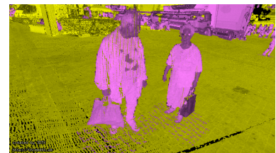
Figure 4.1: Non-static points are identified (magenta)...
