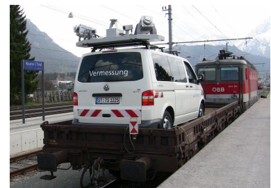
Figure 3.14: The Optech Lynx Mobile Mapper on the back of a train wagon.
